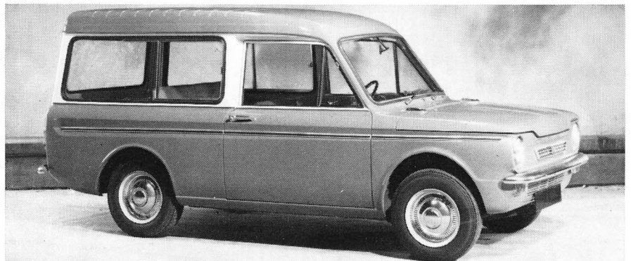
THIS REAR-engined car, the new Hillman Husky, displays the profile of a front-engined car. Slanted sohc engine installation permits cargo deck to be only 27 in. above road level. Fuel tank, spare tire and wheel, and a small additional luggage space are located forward.
