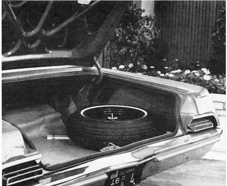
A COULD-BE cavernous cargo compartment was rendered much less spacious by wasteful positioning of spare tire, wheel and tire-change tools.
