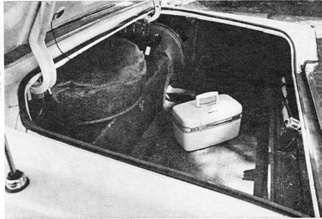
PLACEMENT OF spare, fuel tank location, unusual depth contribute to optimum cargo space utility.
