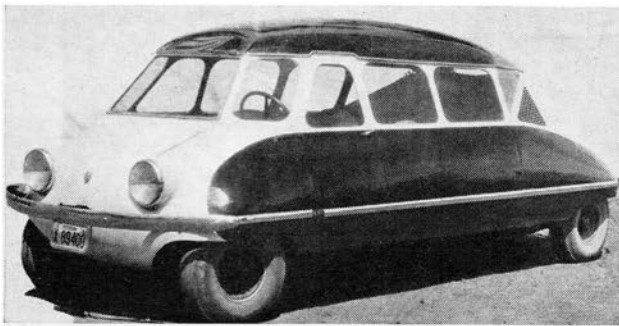
AERODYNAMIC design went into aluminum skinned Scarab No. 1.
